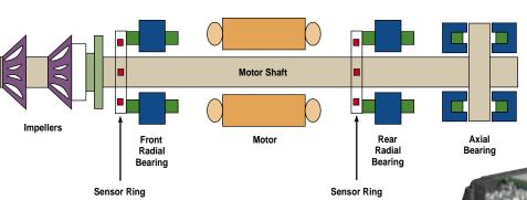
Magnetic bearings and sensors keep the shaft properly centered and positioned at all times.
